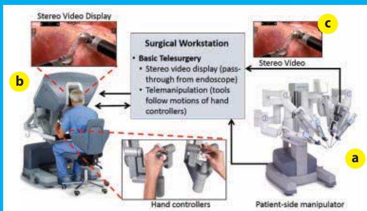
**FIGURE 1** The da-Vinci Si system: (a) the patient side manipulator, (b) the surgeon master interface, (c) the correspondence between dexterous tool wrists and the master interface.
