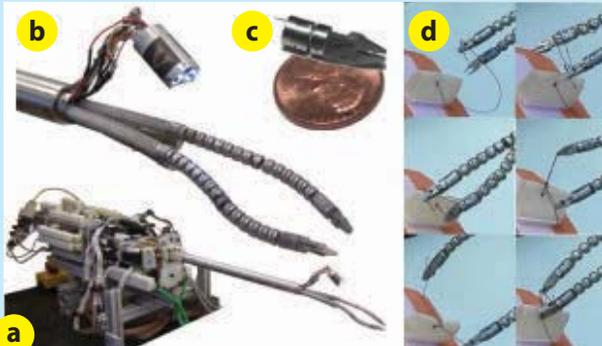
**FIGURE 3** (a) The IREP single port access system, (b) the stereo-vision head with two seven degrees of freedom arms, (c) the distal wrist and gripper, (d) example of tying a double-throw knot.
