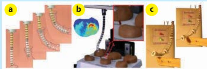
**FIGURE 7** Continuum robots with intrinsic sensing capabilities demonstrating (a) active compliance to facilitate insertion [12], (b) palpation [13], (c) contact detection and localization [11].
